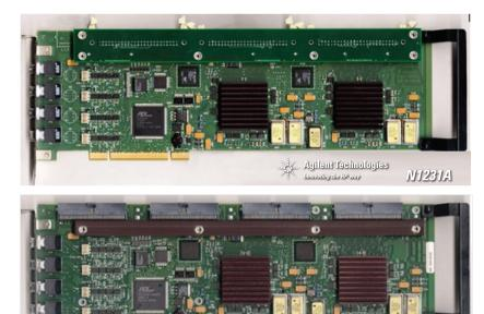
Agilent N1231A/B PCI Three-Axis Laser Axis Boards.
